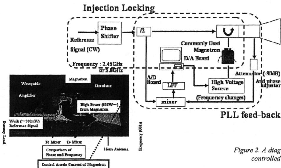
Figure 2. A diagram of the phase-controlled magnetron
