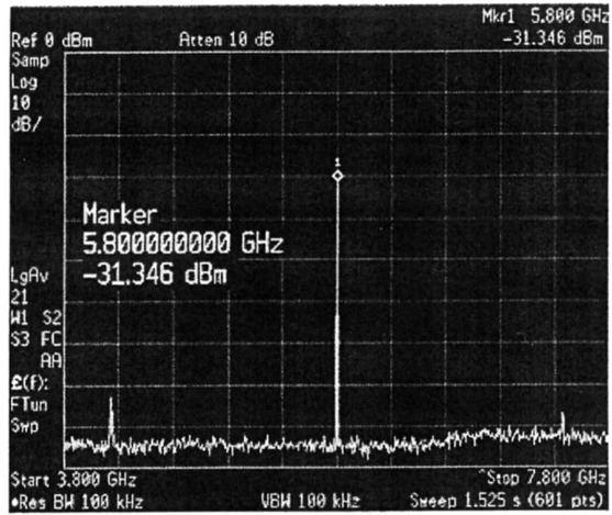
Figure 6b. The output spectrum of the semiconductor amplifier of SPORTS-5.8 (the span is 4 GHz).
