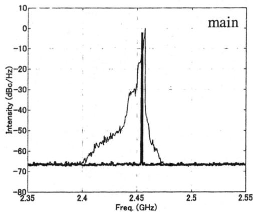
Figure 1. The output spectrum of a commonly used magnetron (bold: with dc-stabilized power supply and filament off; normal: with half-wave voltage-doubler power supply and filament on)
