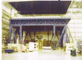
(Image) Near Field XY Scanner (NSI) 12.2m x 6.7m
